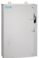
Non-reversing motor starter Size 1 Three phase full voltage Solid-state overload relay OLRelay amp range 0.25-1A 110VAC 50HZ / 120VAC 60HZ coil Combination type 30Amp fusible disconnect 30Amp / 250V fuse clip Encl NEMA type 4X 316 S-steel Water/dust tight non-corrosive Extra-wide enclosure
