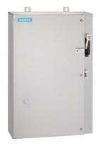
Non-reversing motor starter Size 1 Three phase full voltage Solid-state overload relay OLRelay amp range 0.25-1A 208VAC 60HZ coil Combination type 30Amp fusible disconnect 30Amp / 250V fuse clip Encl NEMA type 4X 316 S-steel Water/dust tight non-corrosive Extra-wide enclosure
