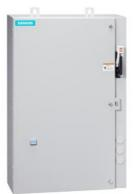
Non-reversing motor starter, Size 1, Three phase full voltage, Solid-state overload relay, OLR amp range 0.25-1A, Combination type, 30A fusible disconnect, 30A/600V fuse clip, Encl NEMA type 4X 304 S-Steel, Water/dust tight noncorrosive, Extra-wide enclosure
