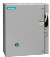
Non-reversing motor starter, Size 1, Three phase full voltage, Solid-state overload relay, OLR amp range 0.25-1A, Combination type, 30A fusible disconnect, 30A/600V fuse clip, Enclosure NEMA type 1, Indoor general purpose use, Extrawide enclosure
