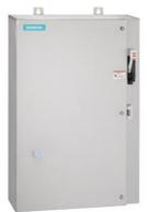
Non-reversing motor starter Size 0 Three phase full voltage Solid-state overload relay OLRelay amp range 5.5-22A 208VAC 60HZ coil Combination type 30Amp fusible disconnect 30Amp / 250V fuse clip Encl NEMA type 4X 316 S-steel Water/dust tight non-corrosive Extra-wide enclosure
