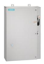
Non-reversing motor starter Size 0 Three phase full voltage Solid-state overload relay OLRelay amp range 3-12A Combination type 30Amp fusible disconnect 30 Amp /600V fuse clip Encl NEMA type 4X 316 S-steel Water/dust tight non-corrosive Extra-wide enclosure
