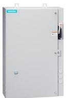
Non-reversing motor starter, Size 0, Three phase full voltage, Solid-state overload relay, OLR amp range 3-12A, 110V 50Hz / 120V 60Hz coil, Combination type, 30A fusible disconnect, 30A/250V fuse clip, Enclosure NEMA type 4/12, Water/dust tight for outdoors, Extra-wide enclosure
