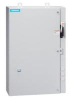
Non-reversing motor starter, Size 0, Three phase full voltage, Solid-state overload relay, OLR amp range 0.75-3.4A, 110V 50Hz / 120V 60Hz coil, Combination type, 30A fusible disconnect, 30A/600V fuse clip, Enclosure NEMA type 4/12, Water/dust tight for outdoors, Extra-wide enclosure
