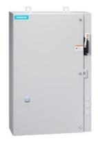
Non-reversing motor starter Size 0 Three phase full voltage Solid-state overload relay OLRelay amp range 0.25-1A 110VAC 50HZ / 120VAC 60HZ coil Combination type 30Amp fusible disconnect 30 Amp /600V fuse clip Enclosure NEMA type 4/12 Water/dust tight weather proof Extra-wide enclosure
