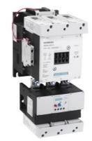
Non-reversing motor starter Size 5 Three phase full voltage Solid-state overload relay OLRelay amp range 55-250A 440-480V 50-60HZ/DC coil Combination type No enclosure
