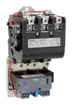
Non-reversing motor starter Size 4 Three phase full voltage Solid-state overload relay OLRelay amp range 50-200A 110-120/220-240VAC 60HZ coil Combination type No enclosure
