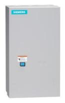
Non-reversing motor starter, Size 3 1/2, Three phase full voltage, Amb. compensate bimetal OLR, Contactor amp rating 115A, 208VAC 60Hz coil, Noncombination type, Enclosure type 1, Indoor general purpose use
