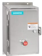
Non-reversing motor starter Size 3 Three phase full voltage Solid-state overload relay OLRelay amp range 25-100A 220-240/440-480VAC 60HZ coil Combination type Water/dust tight non-corrosive
