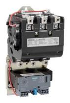
Non-reversing motor starter Size 3 Three phase full voltage Solid-state overload relay OLRelay amp range 25-100A 110VAC 50HZ / 120VAC 60HZ coil Combination type No enclosure
