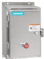
Non-reversing motor starter, Size 2 1/2, Three phase full voltage, Amb. compensate bimetal OLR, Contactor amp rating 60A, 110V 50Hz / 120V 60Hz coil, Non-combination type, Encl. type 4X 304 S. Steel, Water/dust tight noncorrosive
