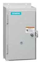
Non-reversing motor starter, Size 2 1/2, Three phase full voltage, Amb. compensate bimetal OLR, Contactor amp rating 60A, 240V 50Hz / 277V 60Hz coil, Non-combination type, Enclosure type 12, Dust/drip proof for indoors
