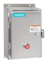
Non-reversing motor starter Size 2 Three phase full voltage Solid-state overload relay OLRelay amp range 13-52a 220-240/440-480VAC 60HZ coil Combination type Water/dust tight non-corrosive
