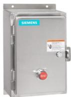
Non-reversing motor starter Size 2 Three phase full voltage Solid-state overload relay OLRelay amp range 13-52a 110-120/220-240VAC 60HZ coil Combination type Water/dust tight non-corrosive
