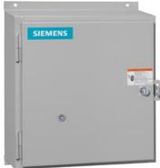
Non-reversing motor starter, Size 2, Three phase full voltage, Solid-state overload relay, OLRelay amp range 13-52a, 550/575 600 50/60HZ coil, Non-combination type, Enclosure type 12, Dust/drip proof for indoors, Extra-wide enclosure
