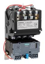
Non-reversing motor starter Size 2 Three phase full voltage Solid-state overload relay OLRelay amp range 13-52a 380-440/440-480V 50/60HZ coil Combination type No enclosure
