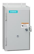
Non-reversing motor starter, Size 2, Three phase full voltage, Solid-state overload relay, OLR amp range 13-52A, Non-combination type, Enclosure type 12, Dust/drip proof for indoors, Standard width enclosure
