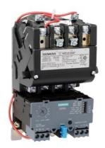
Non-reversing motor starter Size 1 3/4 Three phase full voltage Solid-state overload relay OLRelay amp range 10-40a 190-220/220-240V 50/60HZ coil Combination type No enclosure
