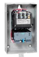
Non-reversing motor starter, Size 1, Three phase full voltage, Solid-state overload relay, OLR amp range 10-40A, 110-120/220-240VAC 60Hz coil, Non-combination type, Enclosure type 1, Indoor general purpose use, Standard width enclosure
