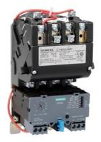
Non-reversing motor starter Size 1 Three phase full voltage Solid-state overload relay OLRelay amp range 3-12A 110-120/220-240VAC 60HZ coil Combination type No enclosure
