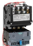
Non-reversing motor starter Size 0 Three phase full voltage Solid-state overload relay OLRelay amp range 5.5-22A 110-120/220-240VAC 60HZ coil Combination type No enclosure
