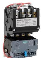
Non-reversing motor starter Size 0 Three phase full voltage Solid-state overload relay OLRelay amp range 3-12A 110-120/220-240VAC 60HZ coil Combination type No enclosure
