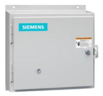
Non-reversing motor starter, Size 0, Single phase full voltage, Solid-state overload relay, OLR amp range 3-12A, 110V 50Hz / 120V 60Hz coil, Non-combination type, Enclosure type 12, Dust/drip proof for indoors, Standard width enclosure
