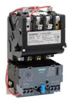
Non-reversing motor starter Size 0 Three phase full voltage Solid-state overload relay OLRelay amp range 0.75-3.4A 380-440/440-480V 50/60HZ coil Combination type No enclosure
