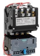
Non-reversing motor starter Size 0 Three phase full voltage Solid-state overload relay OLRelay amp range 0.75-3.4A 110-120/220-240VAC 60HZ coil Combination type No enclosure
