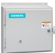
Non-reversing motor starter, Size 0, Three phase full voltage, Solid-state overload relay, OLR amp range 0.75-3.4A, Non-combination type, Enclosure type 12, Dust/drip proof for indoors, Standard width enclosure
