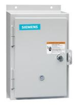
Non-reversing motor starter, Size 0, Three phase full voltage, Solid-state overload relay, OLRelay amp range 0.25-1a, 110 120/220 240VAC 60HZ coil, Non-combination type, Enclosure type 12, Dust/drip proof for indoors, Extra-wide enclosure
