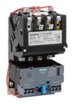
Non-reversing motor starter Size 0 Three phase full voltage Solid-state overload relay OLRelay amp range 0.25-1A 110-120/220-240VAC 60HZ coil Combination type No enclosure
