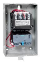
Non-reversing motor starter Size 00 Three phase full voltage Solid-state overload relay OLRelay amp range 3-12A 110VAC 50HZ / 120VAC 60HZ coil Combination type Indoor general purpose use
