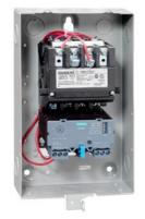
Non-reversing motor starter Size 00 Three phase full voltage Solid-state overload relay OLRelay amp range 3-12A 208VAC 60HZ coil Combination type Indoor general purpose use
