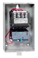
Non-reversing motor starter, Size 00, Three phase full voltage, Solid-state overload relay, OLR amp range 3-12A, Non-combination type, Enclosure type 1, Indoor general purpose use, Extra-wide enclosure
