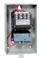
Non-reversing motor starter, Size 00, Three phase full voltage, Solid-state overload relay, OLR amp range 3-12A, 110V 50Hz / 120V 60Hz coil, Non-combination type, Enclosure type 1, Indoor general purpose use, Standard width enclosure
