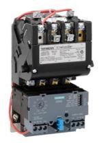
Non-reversing motor starter Size 00 Three phase full voltage Solid-state overload relay OLRelay amp range 3-12A 24VAC 50-60HZ coil Combination type No enclosure
