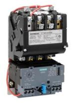
Non-reversing motor starter Size 00 Three phase full voltage Solid-state overload relay OLRelay amp range 3-12A 110-120/220-240VAC 60HZ coil Combination type No enclosure
