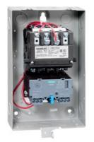
Non-reversing motor starter Size 00 Three phase full voltage Solid-state overload relay OLRelay amp range 0.25-1A 110VAC 50HZ / 120VAC 60HZ coil Combination type Indoor general purpose use
