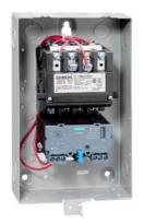
Non-reversing motor starter, Size 00, Three phase full voltage, Solid-state overload relay, OLR amp range 0.25-1A, 240V 50Hz / 277V 60Hz coil, Non-combination type, Enclosure type 1, Indoor general purpose use, Standard width enclosure
