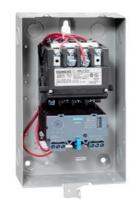
Non-reversing motor starter, Size 00, Three phase full voltage, Solid-state overload relay, OLR amp range 0.25-1A, 24VAC 50-60Hz coil, Non-combination type, Enclosure type 1, Indoor general purpose use, Standard width enclosure
