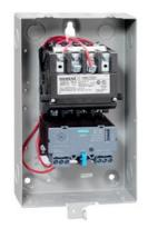
Non-reversing motor starter, Size 00, Three phase full voltage, Solid-state overload relay, OLR amp range 0.25-1A, Non-combination type, Enclosure type 1, Indoor general purpose use, Standard width enclosure
