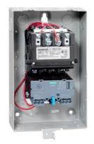
Non-reversing motor starter, Size 00, Three phase full voltage, Solid-state overload relay, OLR amp range 0.25-1A, 110V 50Hz / 120V 60Hz coil, Non-combination type, Enclosure type 1, Indoor general purpose use, Standard width enclosure
