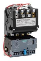
Non-reversing motor starter Size 00 Three phase full voltage Solid-state overload relay OLRelay amp range 0.25-1A 24VAC 50-60HZ coil Combination type No enclosure
