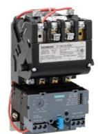
Non-reversing motor starter, Size 00, Three phase full voltage, Solid-state overload relay, OLRelay amp range 0.25-1a, 380 440/440 480V 50/60HZ coil, Non-combination type, Enclosure type (open), No enclosure
