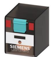
Plug-in relay, 3 changeover contacts 230 V AC, 10 A, Width 22.5 mm for LZS sockets
