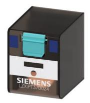
Plug-in relay, 3 changeover contacts 24 V DC, 10 A, Width 22.5 mm for LZS sockets
