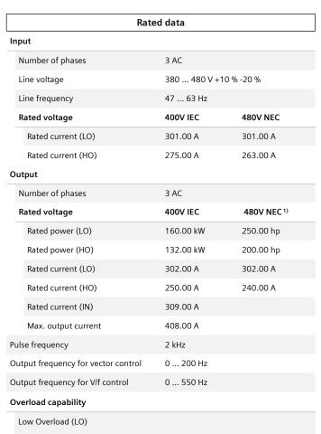
110% base load current IL for 60 s in a 300 s cycle time
