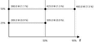
The percentage values show the losses in relation to the rated apparent power of the converter.
