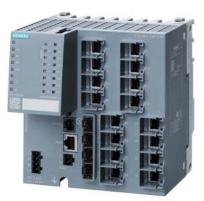
SCALANCE XM416-4C; managed modular IE switch; 16x 10/100/1000 Mbit/s RJ45; 4x 100/1000 Mbit/s SFP; contains 4 combo ports; in total 16 ports can be used; expandable to 24 ports electrical or optical; assembly: DIN rail/S7 mounting rail, PROFINET IO device; redundancy functions; office features (RSTP, VLAN, IGMP,...); C-PLUG in scope of supply; Layer 3 integrated;
